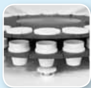
Placing and removing the crucible lids during analysis
