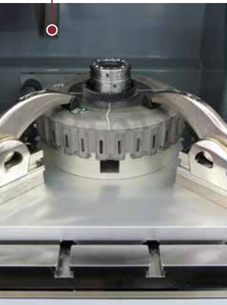
Special clamping device for clutch case
