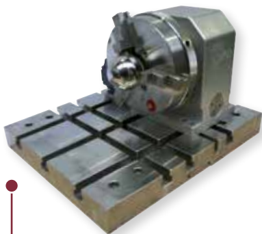
Rotating device with quick changing system
