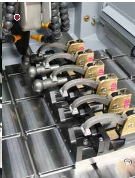
Clamping system for serial cuts of ball heads
