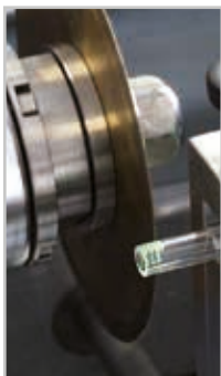
Serial cuts with Z-axis
