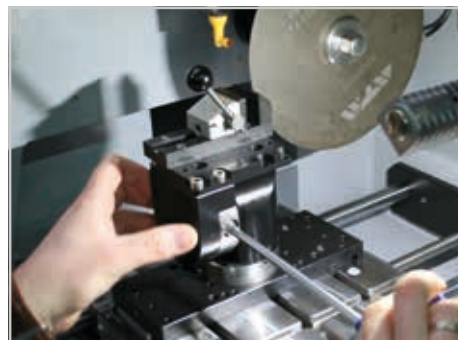
Flexible by rotating and clamping elements
