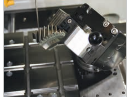
Extension of the pivotal dimension by several rotatable plates
