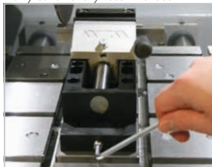
Change of preassembled Easy-clamping bases
