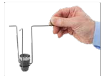
Standard wire crucible holder shown with crucible & lid (VMF/ASTM)
