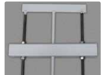
Coal levelling device
