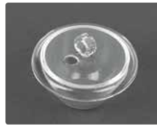
Silica crucible &amp; lid with hole (optional) used for calibration
