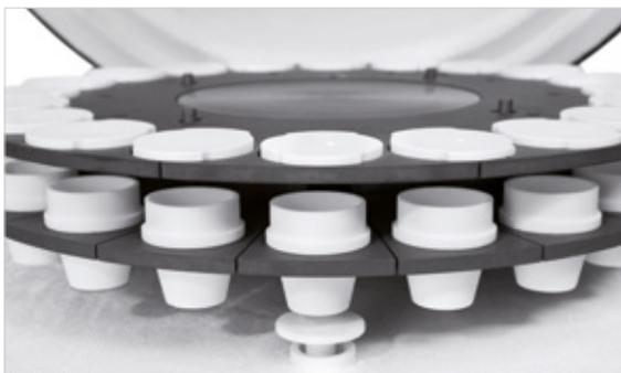
PC-controlled application of crucible lids / crucibles open
