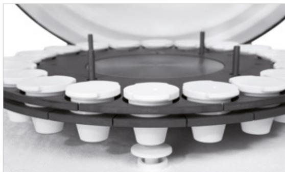
PC-controlled application of crucible lids / crucibles closed
