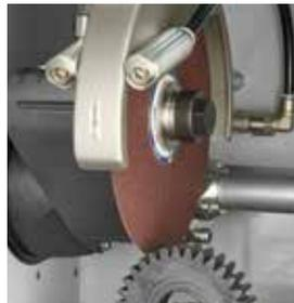
Large cut-off wheel of 254 mm / 10" with parallel moving wheel guard
