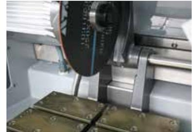
The Qcut 250 M is an especially user-friendly wet abrasive cut-off machine with manual cut-off. Opening the machine folds away the hood to the inside so that the whole cutting chamber is easily accessible. The round window opens a wide field of view during the cutting process.
