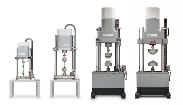
Since 2007, running tests over billions of cycles, ElectroPuls systems are the established materials testing machines using patented linear motor technology. With model capacities up to 20 kN, ElectroPuls systems offer slow-speed static testing and high-frequency dynamic fatigue testing with hundreds of hertz capability.
