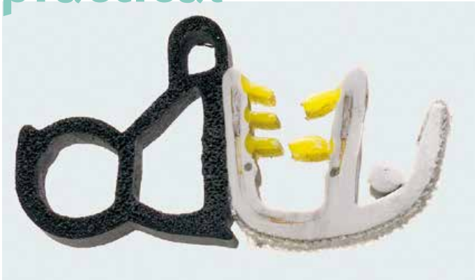
Rubber gasket with metal components: no smearing
