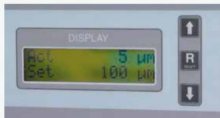
Setting and measurement of grinding removal down to the micron
