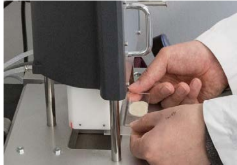
Vacuum head to fix specimen slide
