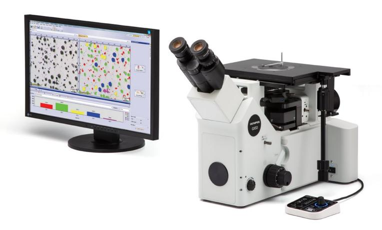
The GX53 inverted microscope is used for a wide range of applications often seen in the steel, automotive, electronics, and other manufacturing industries. The microscope enables users to inspect polished metals and cross-section samples simply by placing them upside down on the stage. The sample does not need to be leveled and can be thick, large, or heavy.
