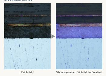
MIX observation combines brightfield and darkfield illumination methods, showing both the sample's color and structure.
