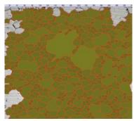
Grain sizing planimetric solution
