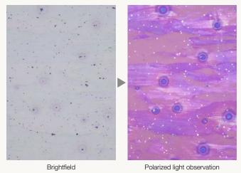
Polarized light observation represents a material's texture and crystal condition brightly. It is suitable for metallurgical structures such as the growth pattern of graphite on nodular cast iron and minerals.
