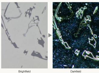
Brightfield is a common observation method to observe reflected light from a sample by illuminating it straight on.
