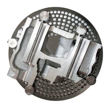
Samples with big dimensions or complicated geometries which normally need manual preparation can be fixed with the universal sample holder for automatic grinding and polishing.
