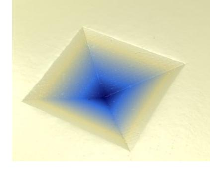
The resulting load-displacement curves are used to calculate hardness and elastic modulus, among other things.
