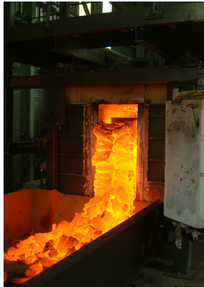
Moving wall coke oven discharging.
