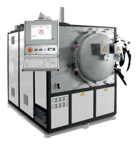
The strong advantage of this approach is the possibility to switch the direction of the gas flow from inside the retort to outside the retort during the process. Hence, the obtained metal parts feature advanced properties. **Carbolite Gero's HTK furnaces can be adjusted to the specific requirements of the MIM process.**
