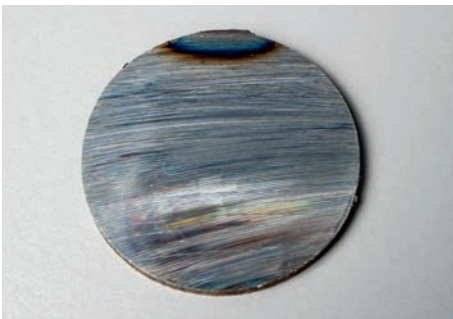
Figure 42: Incorrectly cut sample
