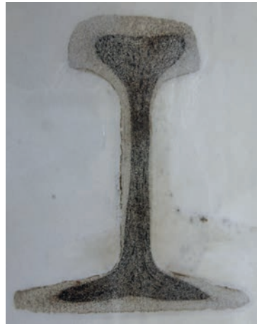
Figure 242: Rail cross-section – Baumann print
