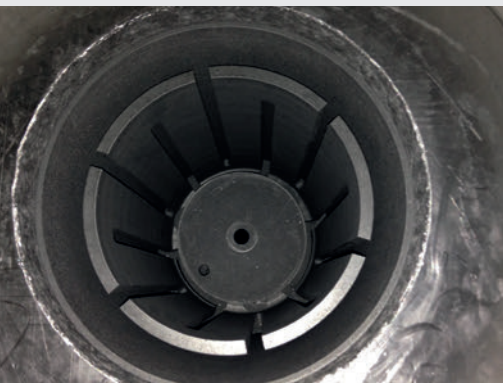
Fig. 15: View from above onto the circular heater of the LHTG furnaces, here with central gas outlet in the middle of the bottom
