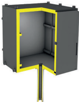
Fig. 8: Schematic view into a retort in a HTK furnace with central gas outlet trough the bottom of the retort
